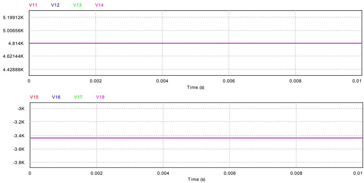
**Figure 11:** Simulation of review circuit in figure 7, using the PSIM software. Note that the unit of perpendicular axes is [V]. The upper figure implies positive electric potentials with the 4 probes along the loop, whereas the lower figure indicates negative electric potentials with the 4 probes in the review circuit along the other loop. As shown, each loop has a uniform electric potential, which satisfies a condition of superconductivity.
