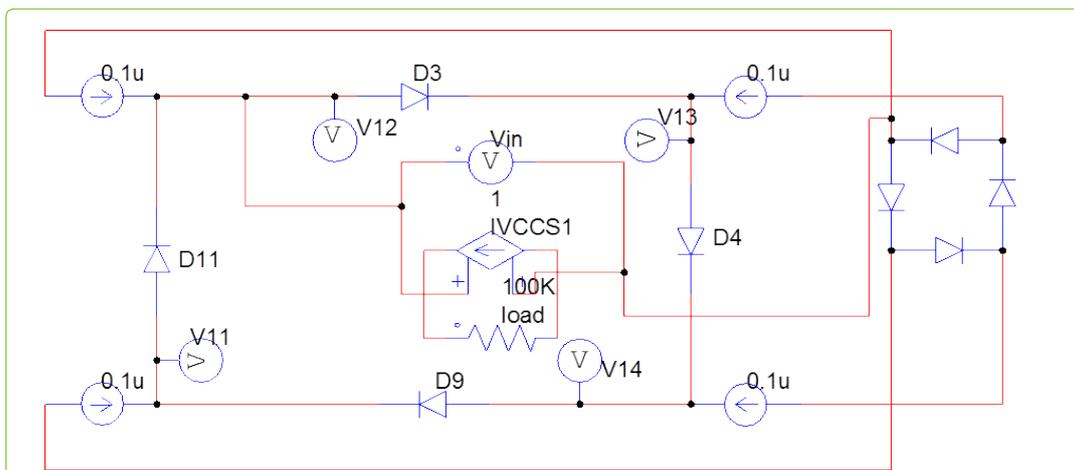
**Figure 9:** The developed circuit, based on the original review circuit, is presented in figure 7. Here a voltage-controlled current source (named IVCCS1) is added. The input voltage  $V_{in}$  is composed of both a loop undergoing positive electric potential as well as a loop undergoing negative electric potential. The load is assumed to be 100 k $\Omega$ .
