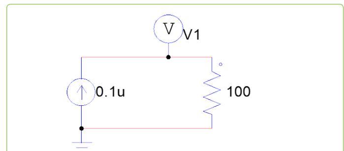
**Figure 8:** An ordinary circuit for comparison with our proposed system circuit (Figure 8). An input current from the current source is 0.1  $\mu$ A, and the load is 100  $\Omega$ . The results regarding the probe V1 are covered in the Results (Section 5)
