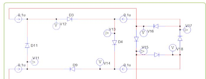
**Figure 7:** Review circuit. The review of our previous work [1] is carried out to better understand the circuits developed in our current paper. Each independent current source inputs 0.1  $\mu$ A. Positive electric potentials are measured by the probes V11–V14, and negative electric potentials are measured by the probes V15–V18.
