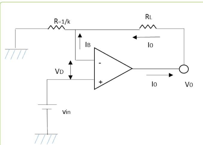
**Figure 2:** Internal configuration of a voltage-controlled current source. This device is a voltage-current converter. Due to the imaginary short of an op-amp,  $V_D$  and  $I_B$  are approximately zero, hence the output current  $I_0$  passing through the load  $R_L$  is determined by the internal conductance  $k$  (i.e.,  $R = 1/k$ ), which is set to 1 in this paper.
