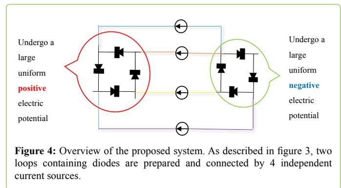
**Figure 4:** Overview of the proposed system. As described in figure 3, two loops containing diodes are prepared and connected by 4 independent current sources.
