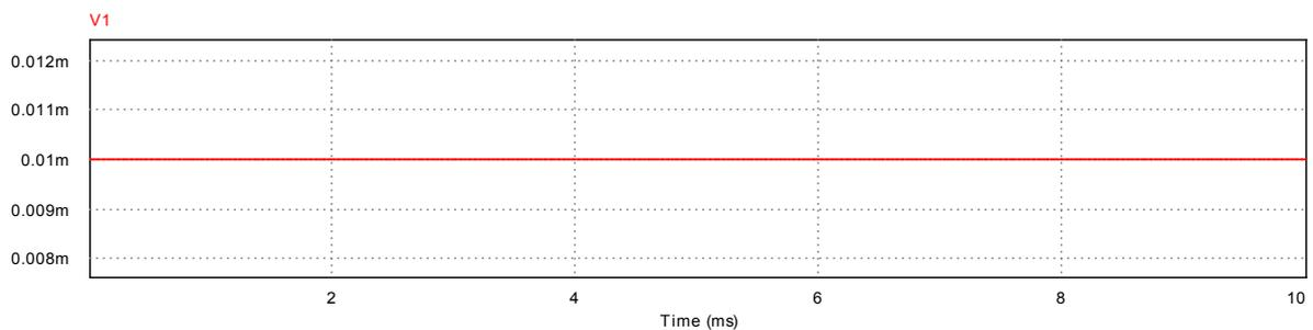
**Figure 12:** The result of an ordinary circuit (shown in Figure 8) in which an independent current source is used, and the load is  $100 \Omega$ . The unit of the perpendicular axis is [V]. Here,  $0.1 \mu\text{A}$  is transmitted to the  $100 \Omega$  load. As shown, the resulting electric potential is small,  $0.01 \text{ mV}$ . In comparison, the proposed system generates kV order for  $0.1 \mu\text{A}$  initial input.
