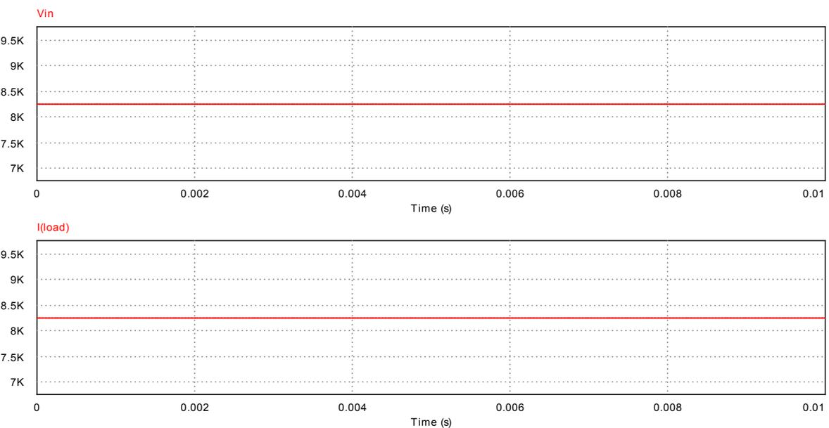
**Figure 13:** Simulation of the circuit upon introducing a voltage-controlled current source (see figure 9). The upper figure indicates the input voltage  $V_{in}$  (the unit is [V]). On the other hand, the lower figure implies the output current with the load (the unit is [A]). An extremely large output current is created because the voltage-controlled current source precisely converted the input voltage.
