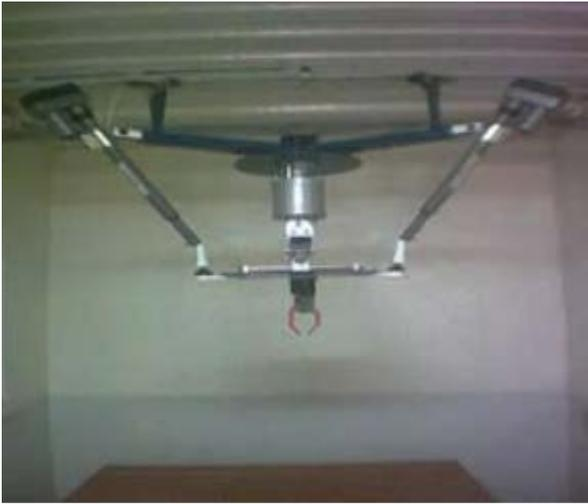
Figure 2: Photo of four-segment constrained parallel robot.
