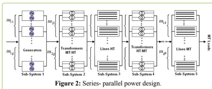
Figure 2: Series- parallel power design.
