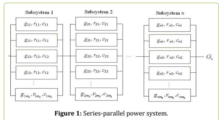
Figure 1: Series-parallel power system.
