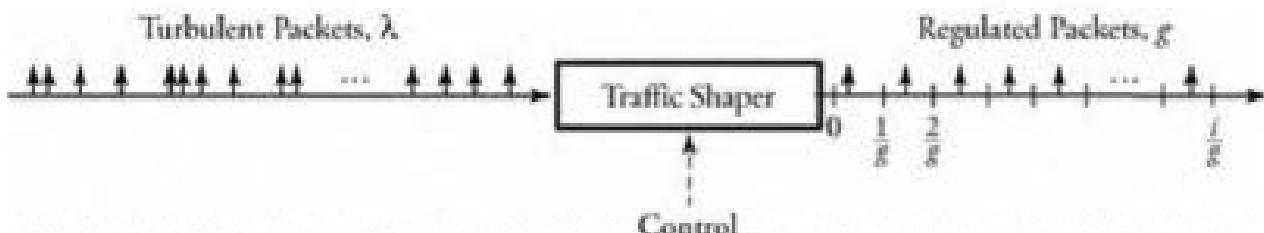
**Figure 1:** How turbulent packets  $\lambda$  are shaped to regulated packets  $g$  source (e-learning atria report).
